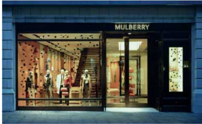
Good vertical illumination helps define the size of the space and can even lead the customer's eye around and deep into the store from outside the shop.
