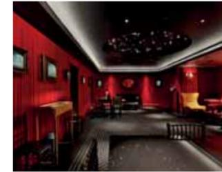
Coves provide opportunities for concealed lighting to provide both ambient and feature light, while simultaneously providing visual interest to the customer.
